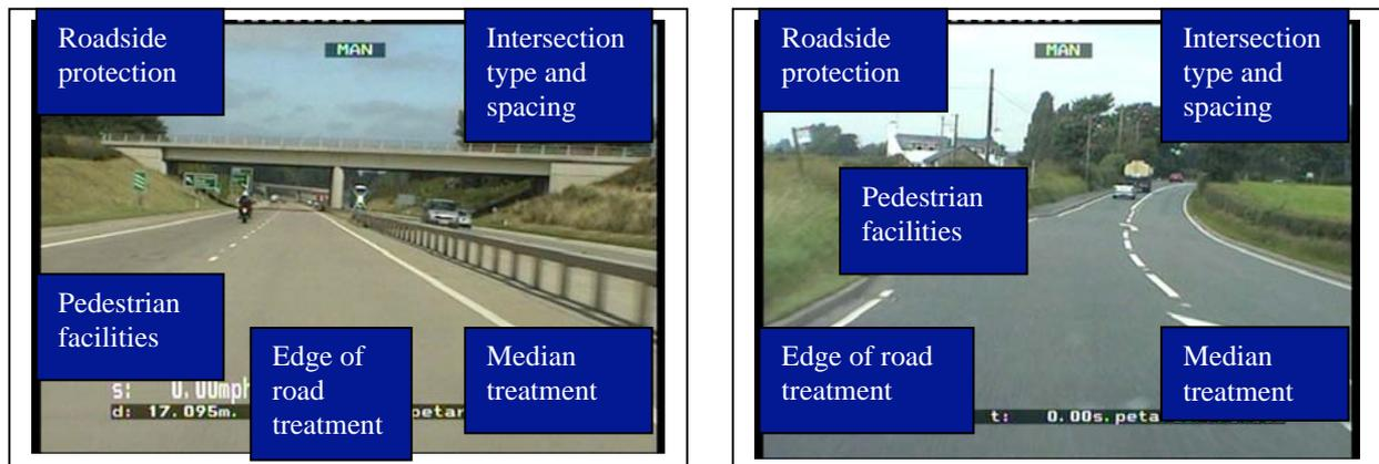
**Figure 14** Areas of road which are inspected for developing the Road Protection Score
