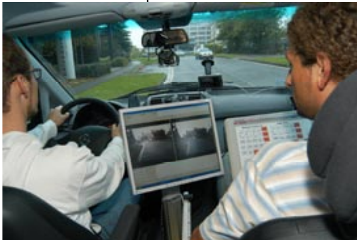
Fig. 7: Inside camera (below rear-view mirror) and monitor for displaying video pictures.
