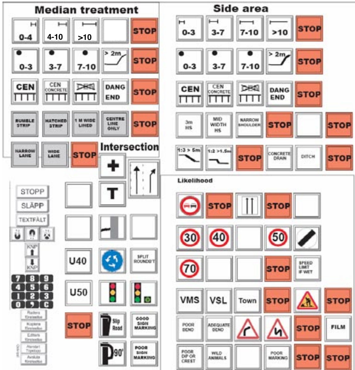
Fig. 3: Overlay of digitising tablet used for RPS inspections in UK
