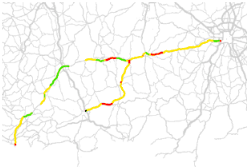
Fig. 5: Presentation of inspection data using ArcGIS from ESRI
